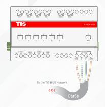
4>> Connect the load (Driver Power) electrical wires to outputs 1-6. Each channel can control up to 10A loads. The installer should make sure not to overload the device and module channels.
