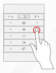
Test the button on the panel by short **3** pressing it for ON/OFF and long pressing it to dim (if channel is dimmable).
