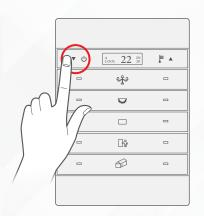
3 D Test your air conditioning by changing the mood, Heat/Cool, and fan speed from low to medium to high. HVAC module should respond accordingly.
