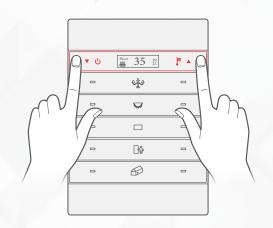
**3** Test your floor heating by changing the temperature, relay should respond accordingly.
