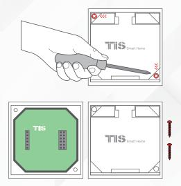
Connect the Wall Base and Panel 4>> Addition in this position. Place the upper pins as shown, and then push the pins down with your fingers to assemble.
