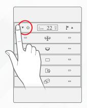
**3** Test your air conditioning by changing the fan speed from low to medium to high. Your relay should respond accordingly.
