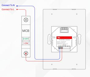
1.5 mm Electric Cable 1.5 mm Electric Cable
