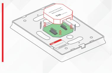
**10** Connect the main Luna panel vertically to the part installed on the wall; install the upper part by making sure the buckles are completely inside.
