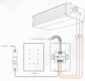
2.5 mm Electric Cable 1.5 mm Electric Cable 1.5 mm Electric Cable GND(white-orange)&(white-brown) D-(white-green)&(white-blue) D+(blue-green) 24+V(brown-orange)
