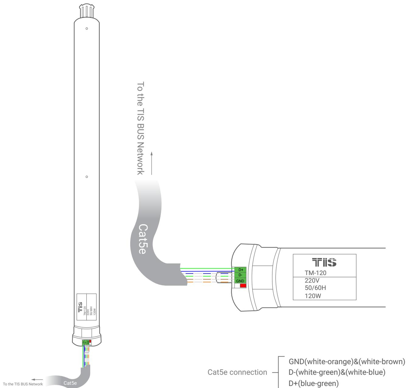
▲ Figure 2: Roller Curtain Motor's BUS Color Coding
