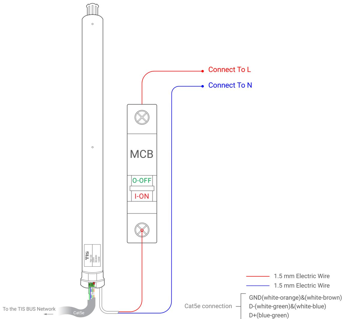
▲ Figure 1: Roller Curtain Motor's Bus Connection Diagram
