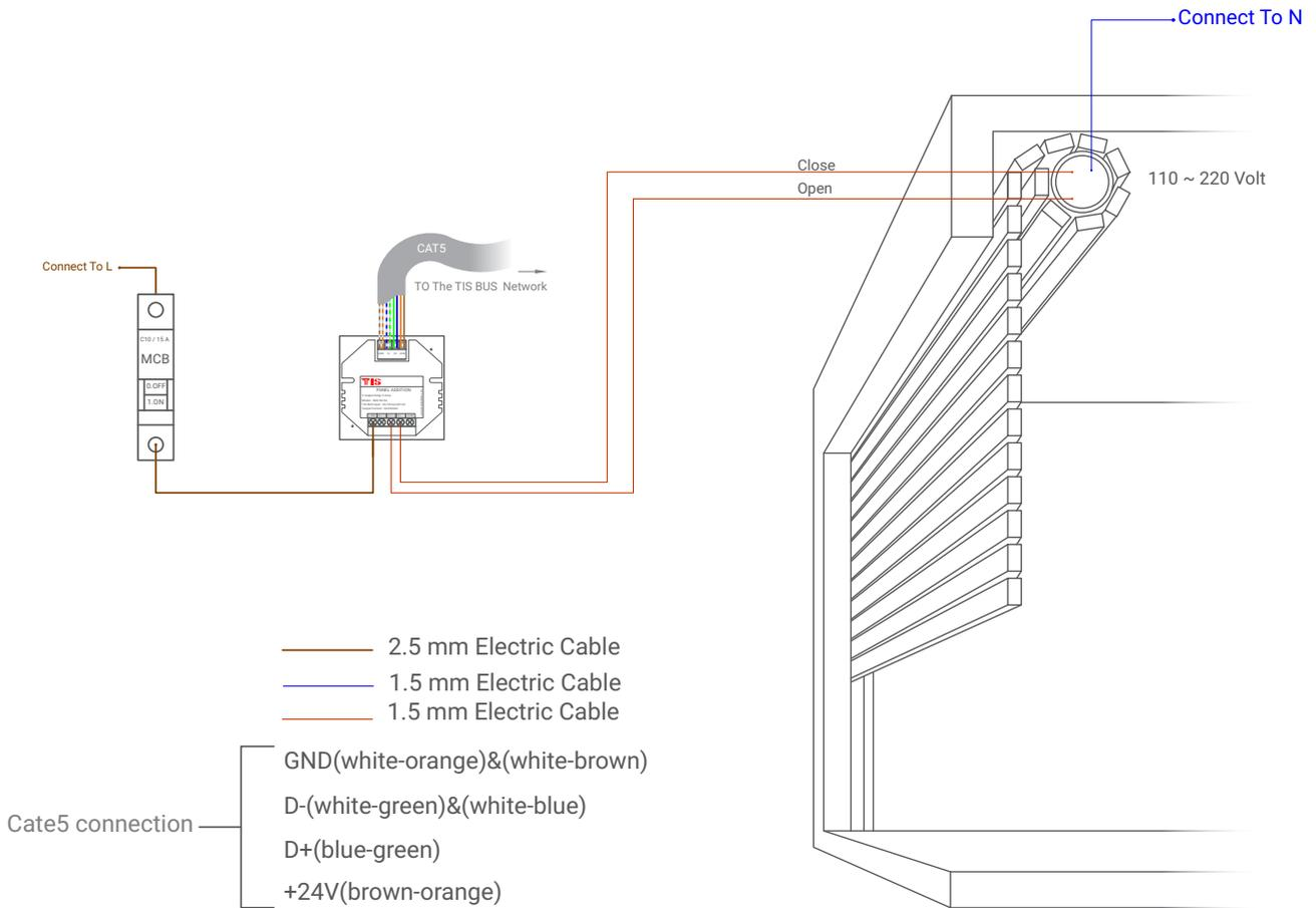
▲ Figure 2: ADD-3R-5A Motors Connection Diagram
