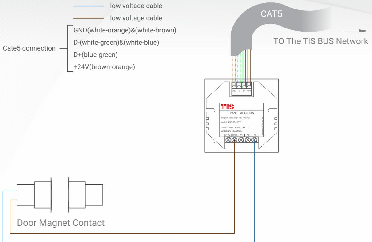
▲ Figure 1: Magnetic Door Contact Connection Diagram
