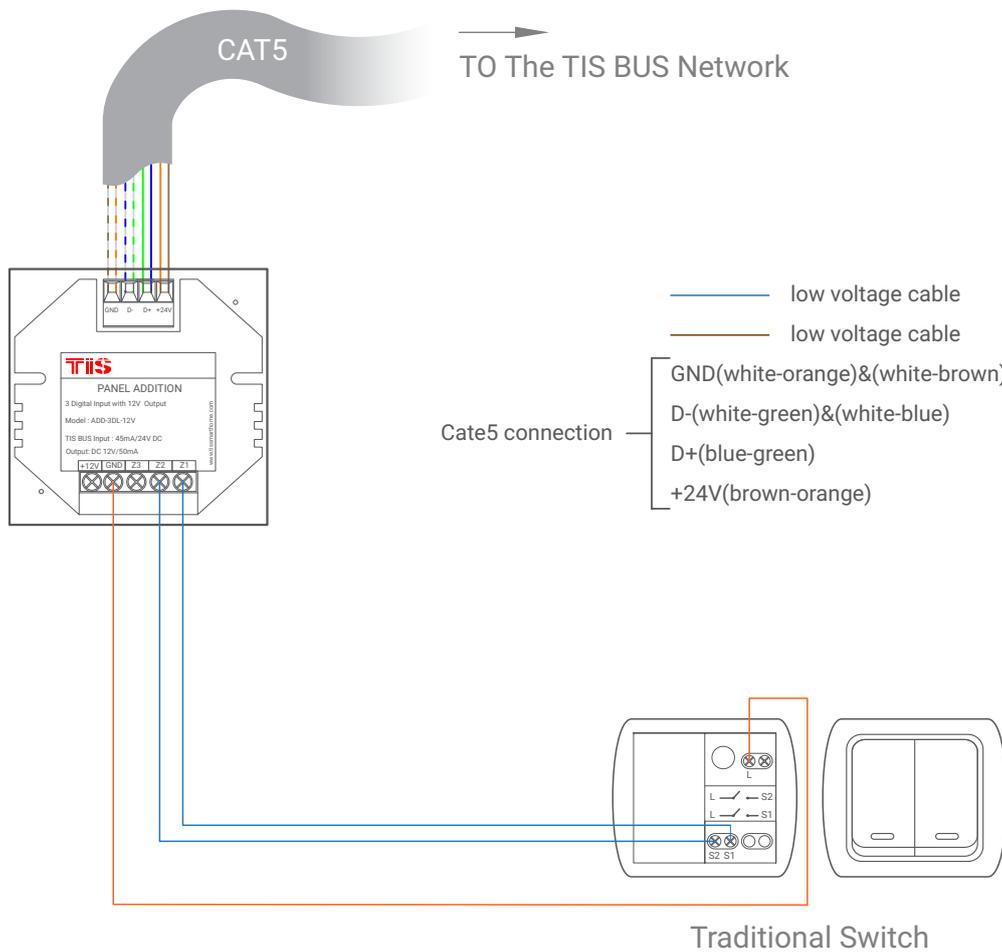
▲ Figure 3: Traditional Switch Connection Diagram
