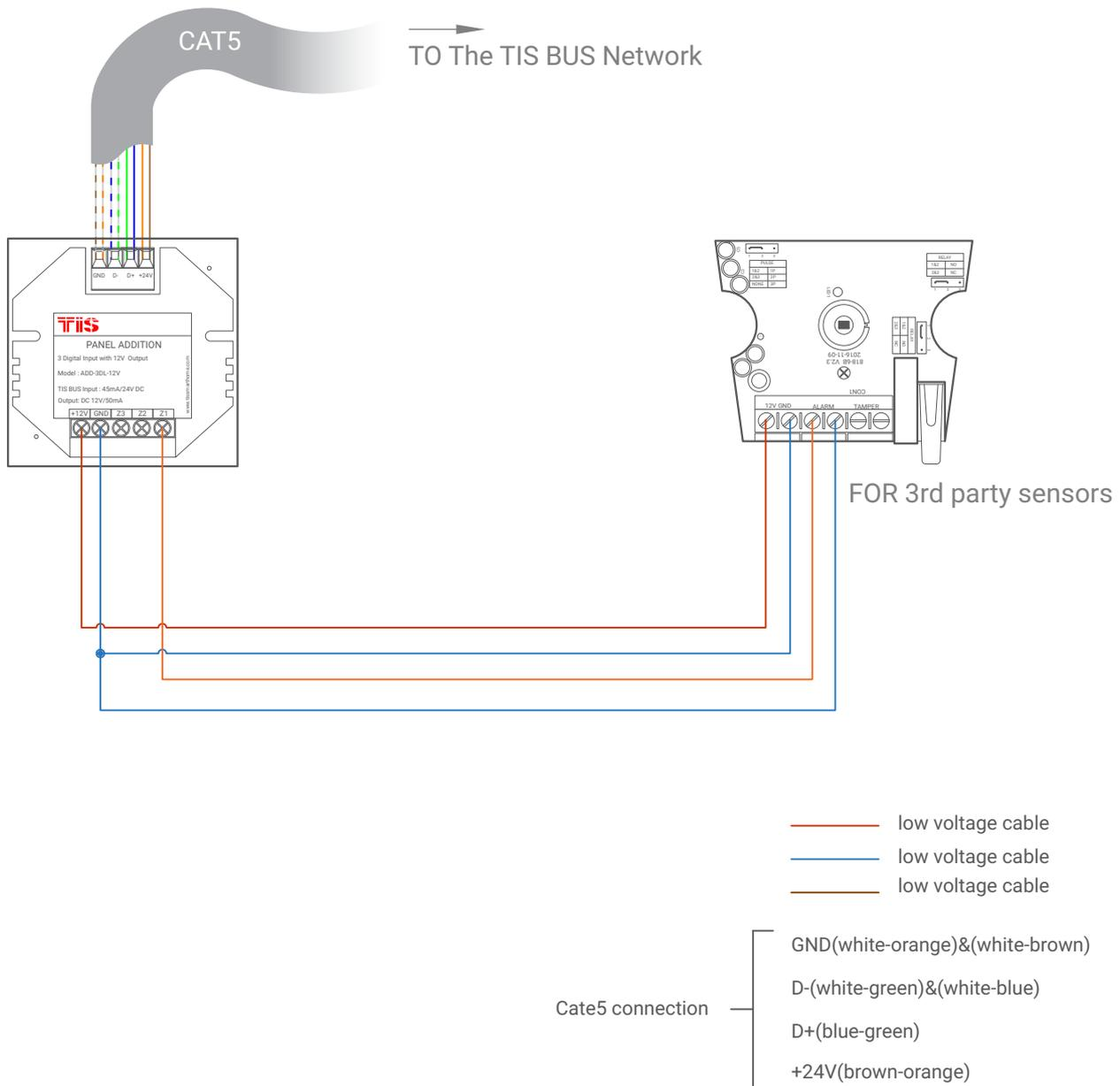
▲ Figure 2: 3<sup>rd</sup> Party Sensor Connection Diagram
