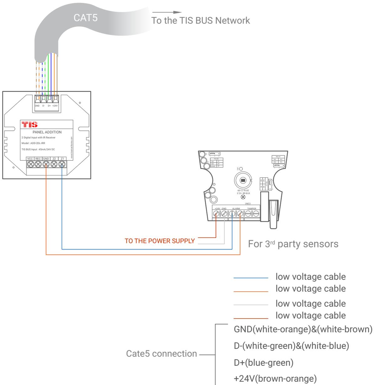
▲ Figure 2: ADD-2DL-IRR & 3<sup>rd</sup> Party Sensor Connection Diagram
