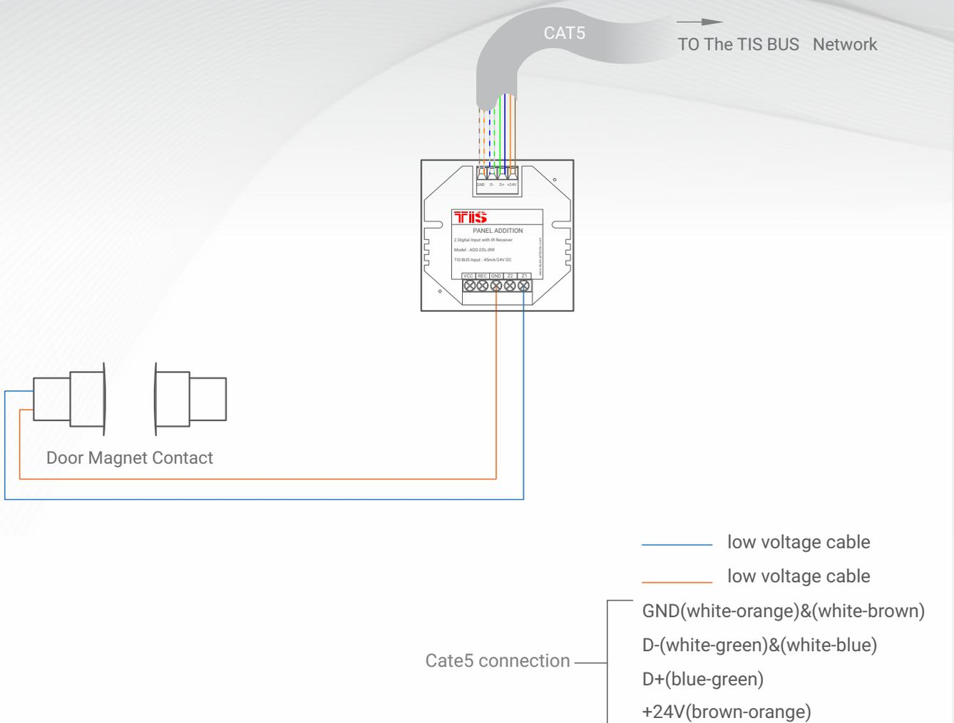
▲ Figure 1: ADD-2DL-IRR & Magnetic Door Contact Connection Diagram
