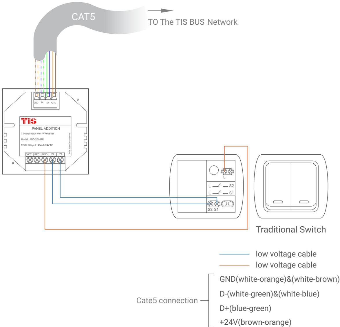
▲ Figure 4: Traditional Switch Connection Diagram
