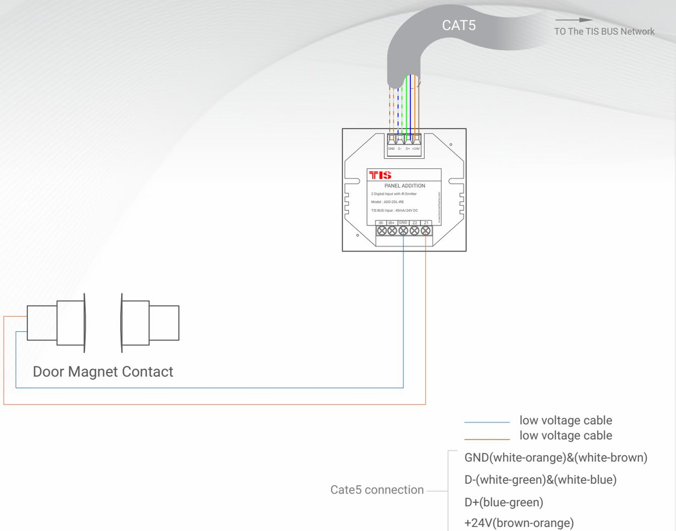
▲ Figure 1: ADD-2DL-IRE & Magnetic Door Contact Connection Diagram
