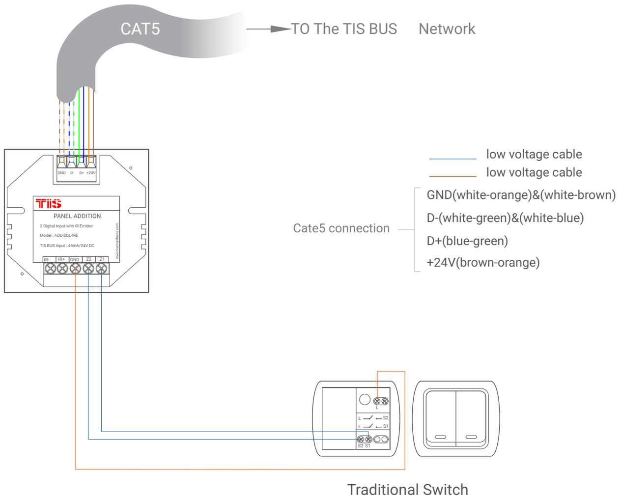
▲ Figure 4: ADD-2DL-IRE & Traditional Switch Connection Diagram
