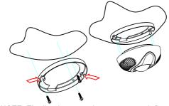
NOTE: The line between the two screws defines the detection of longer sensing range (see the field of view diagram).
