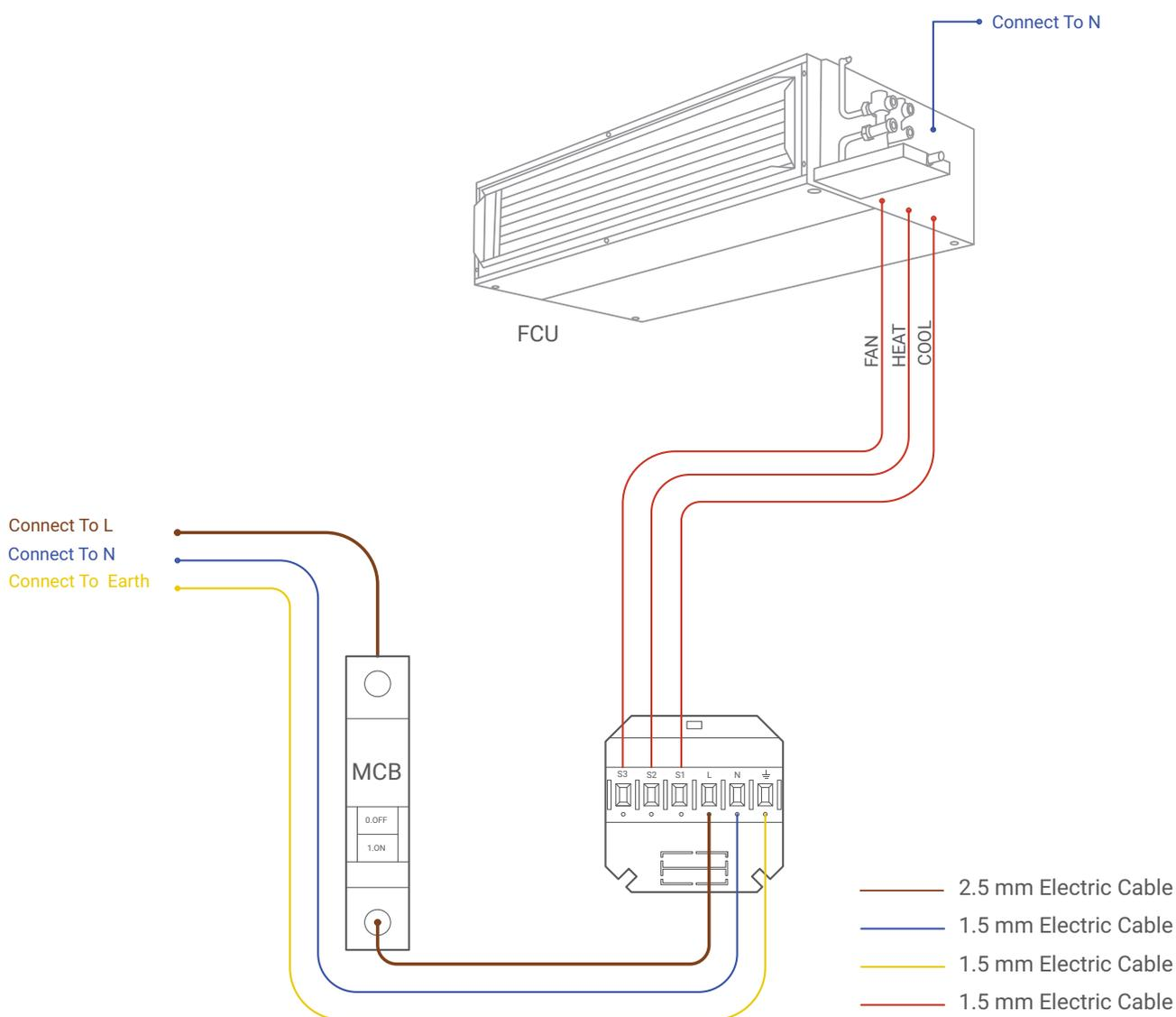
▲ Figure 4: HVAC Connection Diagram
