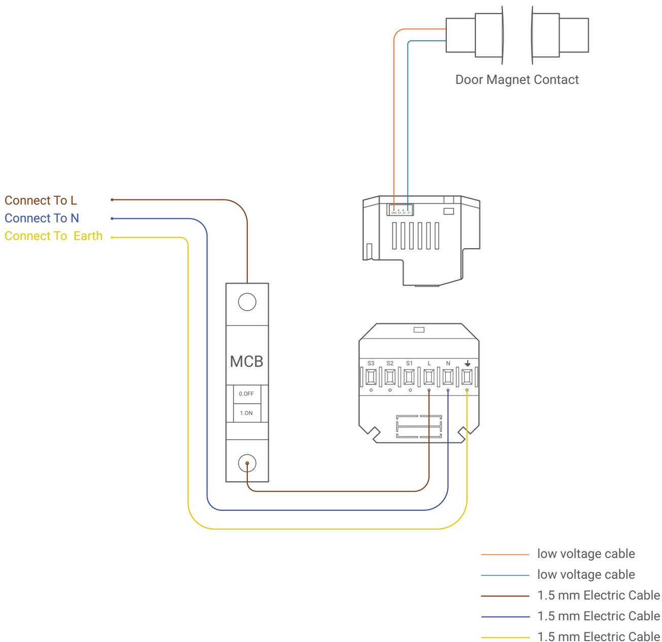
▲ Figure 5: Magnetic Door Contact Connection Diagram
