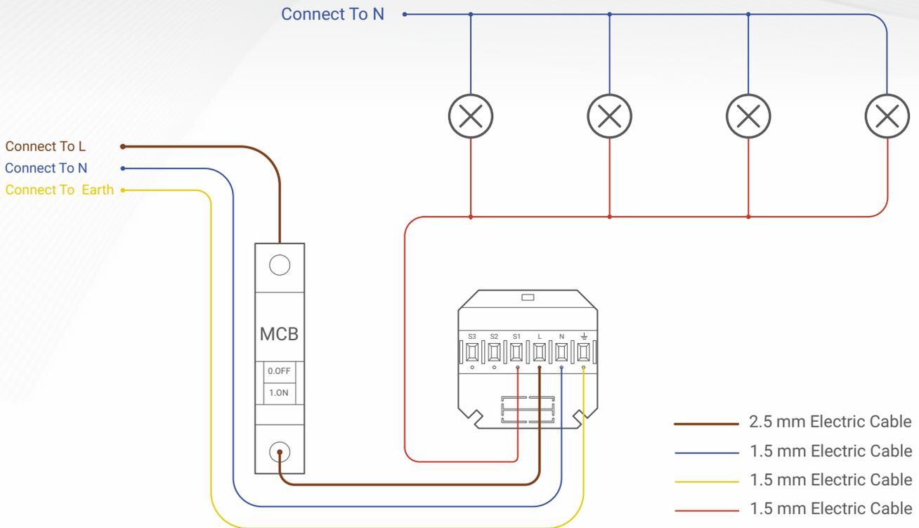
▲ Figure 1: Lights Connection Diagram
