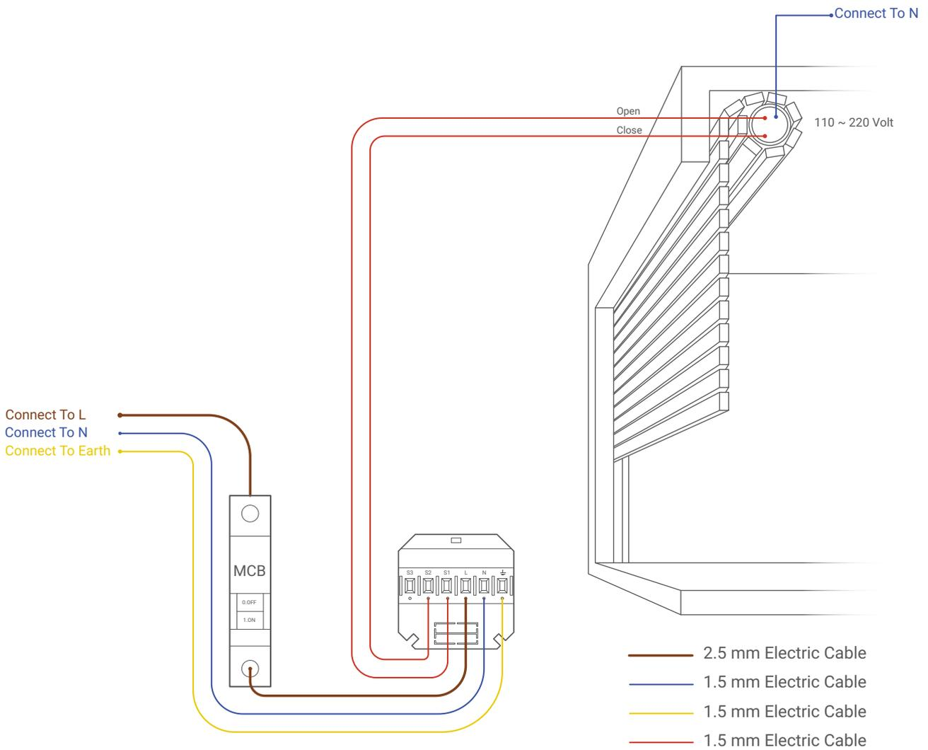
▲ Figure 2: Motors Connection Diagram
