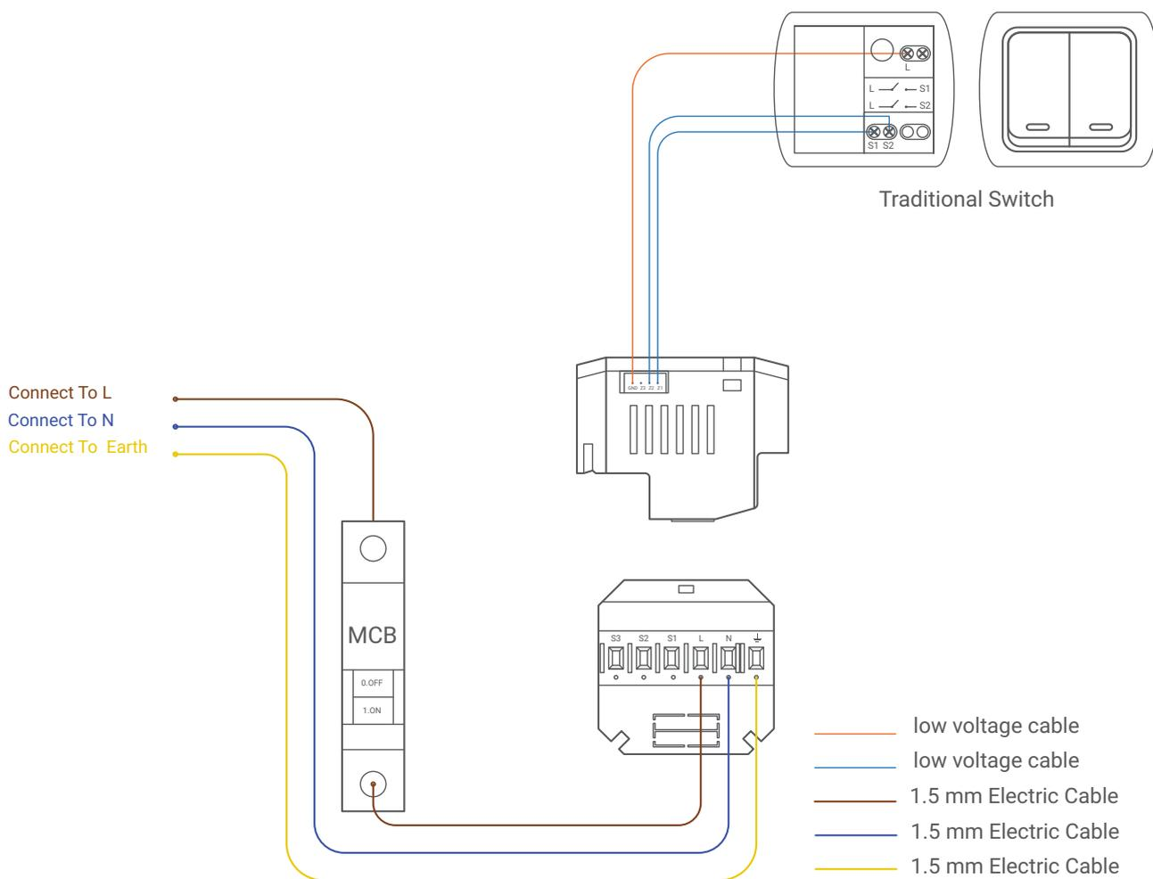
▲ Figure 7: Traditional Switch Connection Diagram
