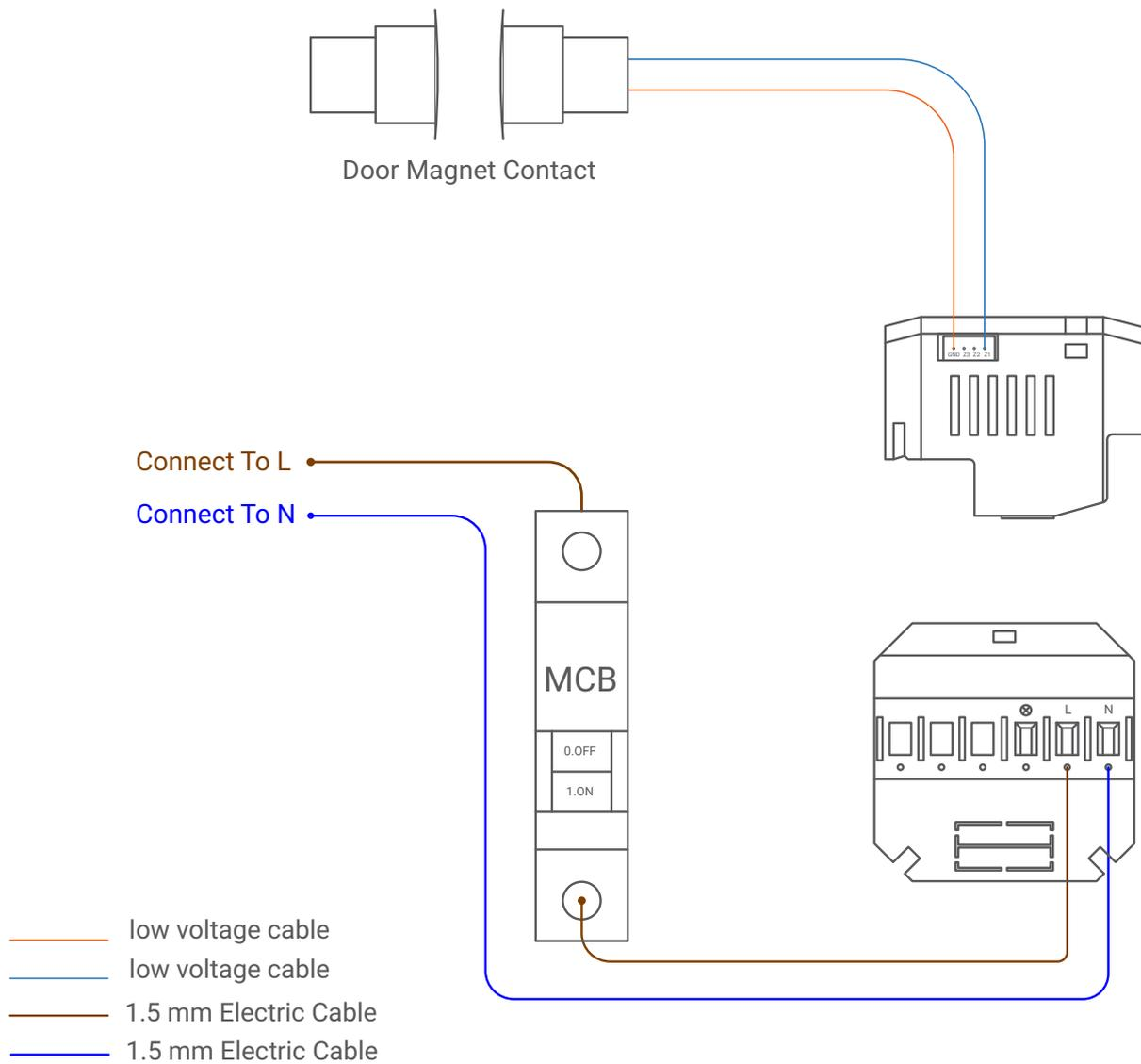
▲ Figure 2: Magnetic Door Contact Connection Diagram
