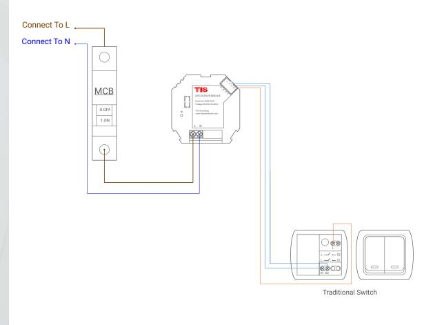
Figure 3: ACM-3Z-IN & Traditional Switch Connection Diagram
