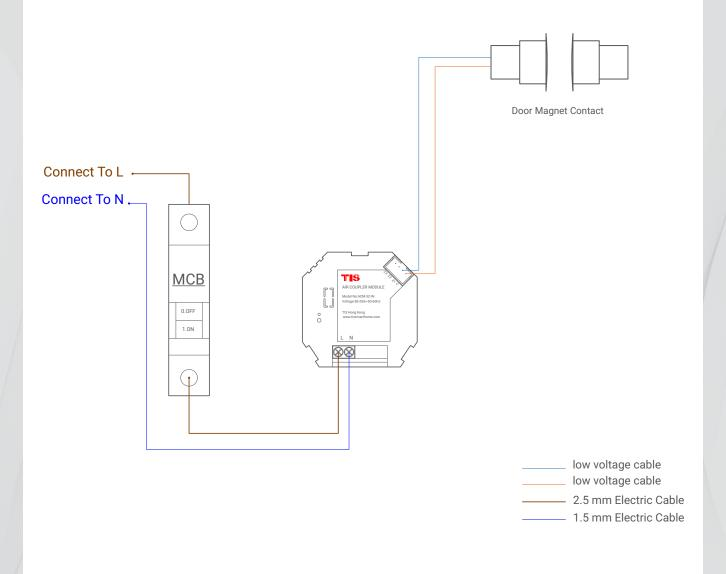
Figure 2: ACM-3Z-IN & Magnetic Door Contact Connection Diagram
