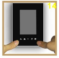
install the upper part make sure the buckles totally inside than push it from down side to be fixed on wall
