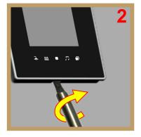
Rotate the screwdriver by 90 degrees.
