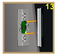
Connect the main Luna panel vertically to the other installed part in the wall
