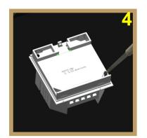
Open the 2 screws on the Panel Addition cover.
